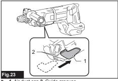
▶ 1. Air duct cap 2. Guide grooves
