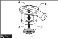
1. Cap 2. Printed side 3. Grooves 4. Lips of upper opening 5. Attachment unit
