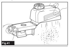
NOTICE: When cleaning the filter, tap the case of the filter gently by hand to remove dust. Do not tap the filter directly; touch the filter with brush or similar; or blow compressed air on the filter. Doing so may damage the filter.
