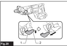
1. Air duct cap 2. Lock tab
