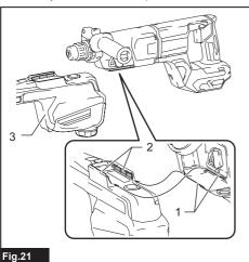
1. Guide grooves 2. Guide rails 3. Dust collection system
