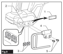
1. Rubber cap 2. Mounting bracket 3. Plate washers 4. Hook 5. Screws
