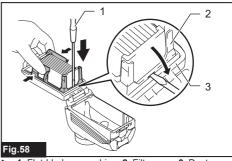
1. Flat-blade screwdriver 2. Filter case 3. Dust case cover
