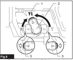
1. Rotation with hammering 2. Action mode changing knob 3. Release button
