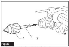
1. Keyless drill chuck 2. Chuck adapter
