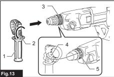
1. Side grip 2. Thumb screw 3. Barrel neck of the gear housing 4. Retaining projection 5. Positioning recess
