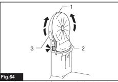
1. Rubber edges 2. Sealing cap 3. Nozzle head
