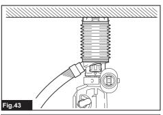
**NOTICE:** Do not use the dust cup set when drilling in metal or similar. It may damage the dust cup set due to the heat produced by small metal dust or similar.
