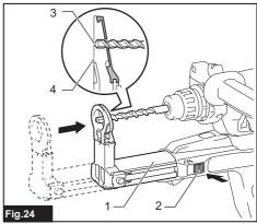
1. Nozzle guide 2. Guide adjustment button 3. Tip of drill bit 4. Front surface of nozzle
