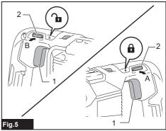
▶ 1. Switch trigger 2. Lock-off button
