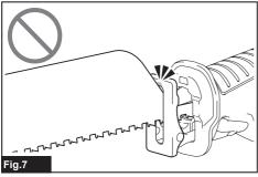
When the recipro saw blade loses its cutting efficiency in one place along its cutting edge, reposition the shoe to utilize a sharp, unused portion of its cutting edge. This will help to lengthen the life of the recipro saw blade.
