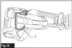
The hook is convenient for hanging the tool temporarily. To use the hook, simply lift up hook until it snaps into the open position.
