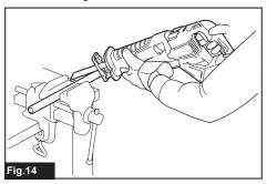
NOTICE: Do not cut the workpiece with the shoe away from the workpiece or without the shoe. Doing so increases the reaction force which may break the recipro saw blade.
