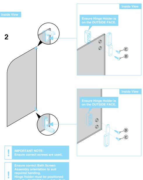
onto the OUTSIDE face of the Bath Screen Assembly.
