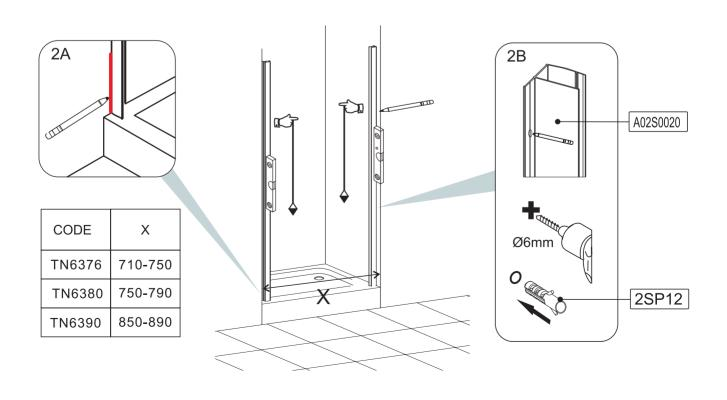
When fitting a fully framed product into a recess you must push the wall profiles onto the uprights. This is done as fitting the wall profiles first in a tight recess may lead to difficulty later when fitting the door.
