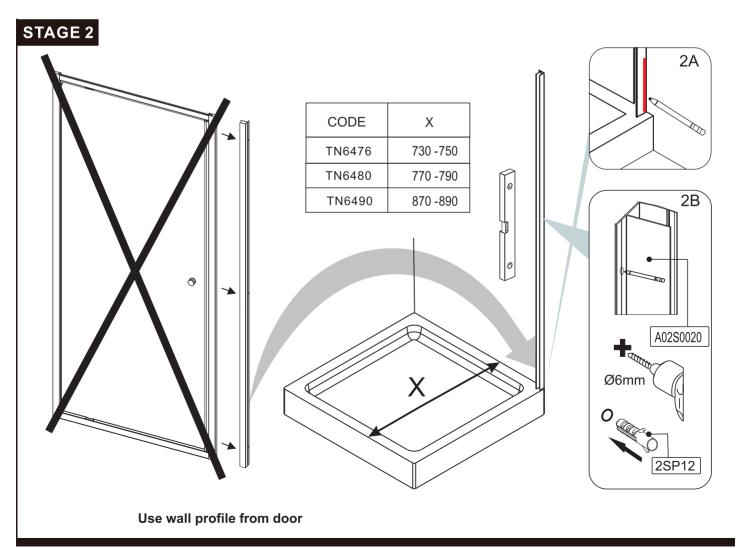
After your wall profiles have been fixed you can square your side panel on the tray and fix the wall profiles to the upright profiles as shown below.
