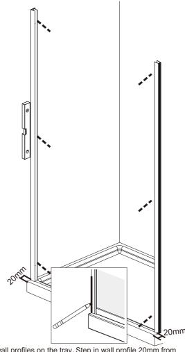
Position the wall profiles on the tray. Step in wall profile 20mm from the front edge of the shower tray. Ensure wall profile is plumb. Mark the position for fixing the wall profile to the wall. Drill with 6mm Masonry drill bit and insert wall plug SP02SP12 Do not silicone behind wall profile to wall, see sealing section.
