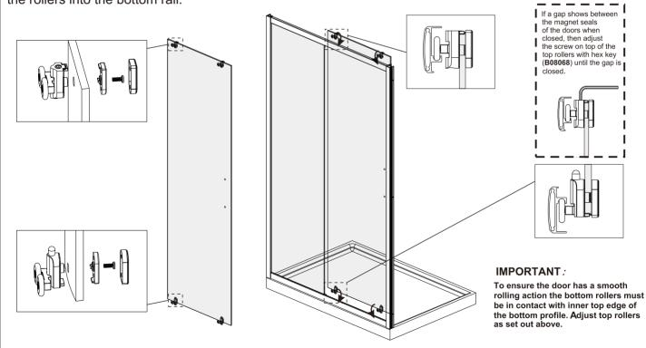
**SECURE WALL CHANNEL & UPRIGHT PROFILE**Once you have check that the door opens and the closes correctly, fix the door frame to the wall channels. From inside, drill 3 holes through each wall channel/door frame using 3.0mm drill bit. Fix using A2401201.
