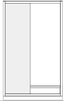
Fit both wall profile onto the frame, then lift the frame onto the tray, keep side of profile with fixing holes to the inside, fix both profiles with 30mm screws A2403001.
