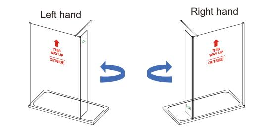
Remove swivel panel from packaging. Install the swivel panel in required orientation. Product is reversible and no brackets need to be removed to change handing.
