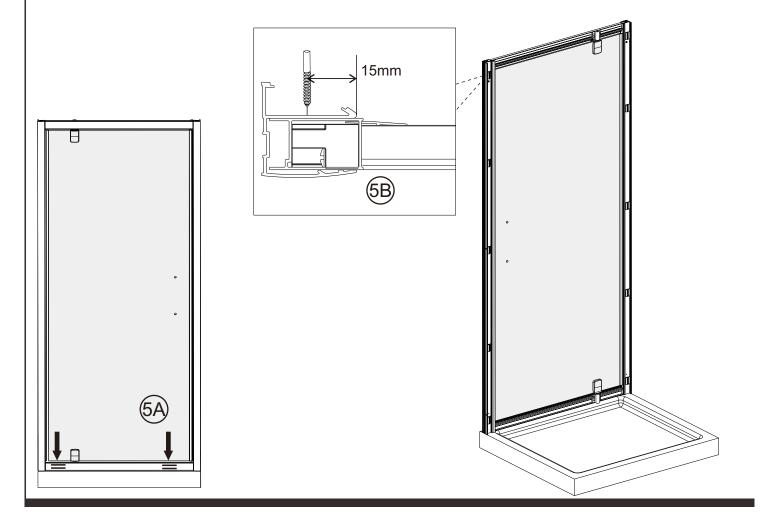
Fix the frame with screws **A2401201**. **IMPORTANT:** Ensure frame is 100% square and the door closes square in the frame ( should be an even gap between bottom of door panel and the bottom profile).
