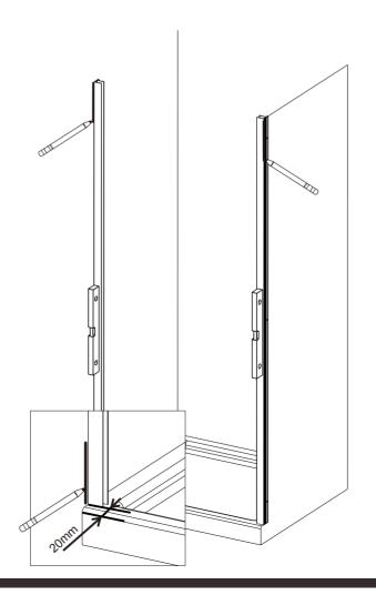
Fit both wall profiles onto the frame, then lift the frame onto the tray. Keep side of profile with fixing holes to the inside, fix both profiles with 30mm screws A2403001.
