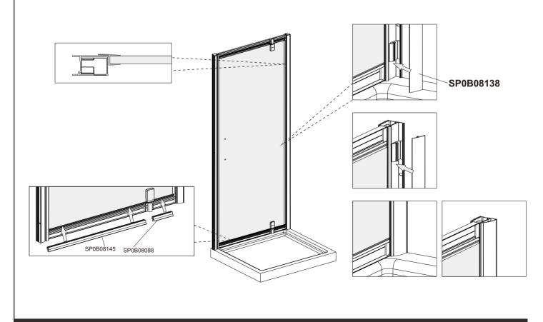
Insert wall profile covercaps **SP0B08150/SP0B08151** followed by the upright profile covercaps **SP0B08152**.Place a dab of silicone on the cover cap legs to
