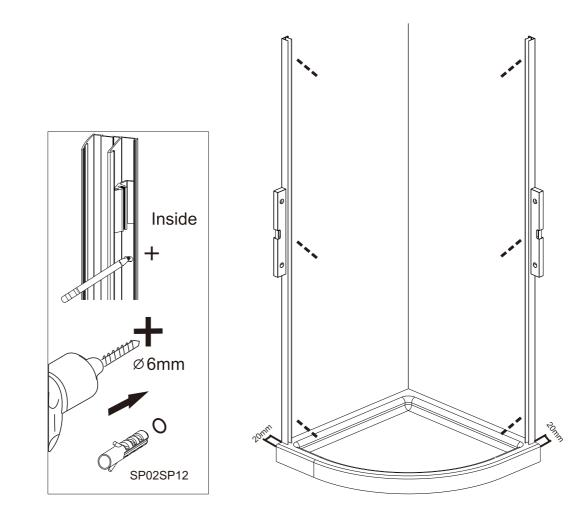
Position the wall profiles on the tray. Step in wall profile 20mm from the front edge of the shower tray. Ensure wall profile is plumb. Mark the position for fixing the wall profile to the wall. Drill with 6mm Masonry drill bit and insert wall plug **SP02SP12 Do not silicone behind wall profile to wall, see sealing section**.
