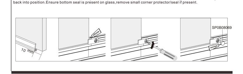
Put a dab of silicone in the corner between glass panel and fixed clip to the bottom when sliding the clip under the glass and
