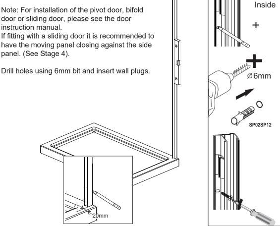
Fix the wall profile to the wall with screws A2403001.
