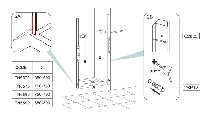
When fitting a fully framed product into a recess you must push the wall profiles onto the uprights. This is done as fixing the wall profiles first in a tight recess may lead to difficulty later when fitting the door.
