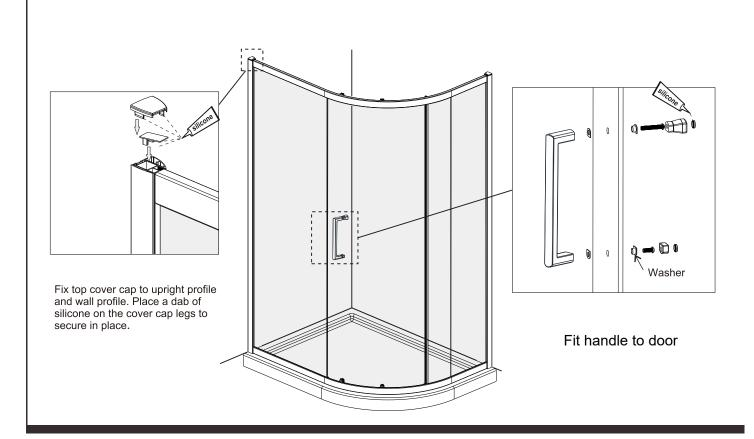
Use a quality silicone sealant to seal the finished door. Seal joints between the upright profiles and the bottom rail. Sealing Inside Seal top to bottom on the INSIDE between the wall profile and the wall. Note :Do not apply sealant on inside of tray.
