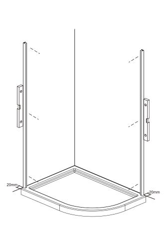
Position the wall profiles on the tray. Step in wall profile 20mm from the front edge of the shower tray. Ensure wall profile is plumb. Mark the position for fixing the wall profile to the wall. Drill with 6mm Masonry drill bit and insert wall plug **SP02SP12 Do not silicone behind wall profile to wall, see sealing section**.
