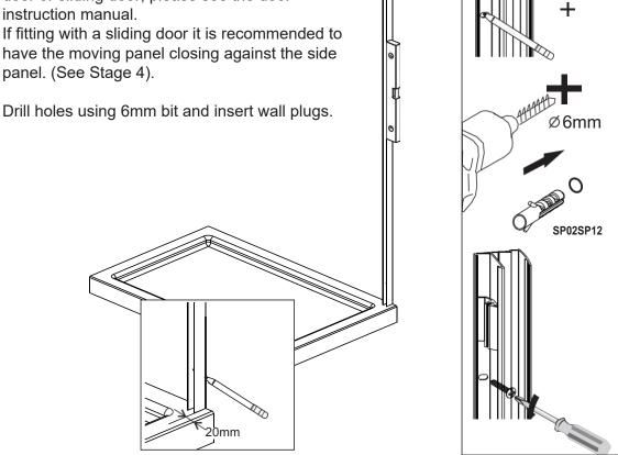
Fix the wall profile to the wall with screws A2403001.
