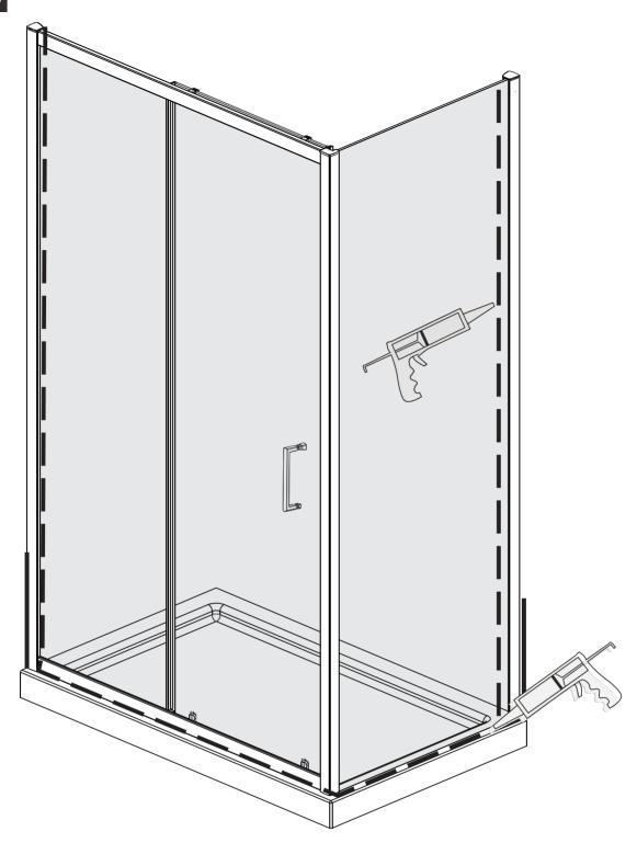
Use a quality silicone sealant to seal the finished door.
