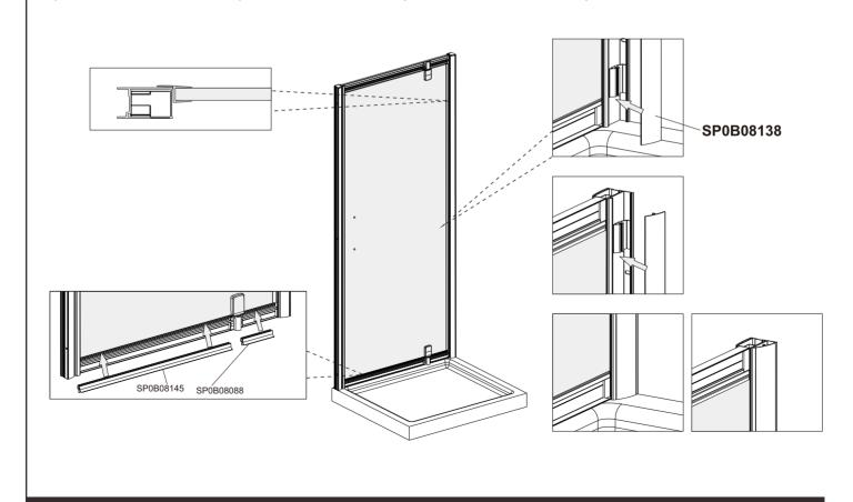
Insert wall profile covercaps **SP0B08150/SP0B08151** followed by the upright profile covercaps **SP0B08152**.Place a dab of silicone on the cover cap legs to
