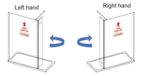
Remove swivel panel from packaging. Install the swivel panel in required orientation. Product is reversible and no brackets need to be removed to change handing.
