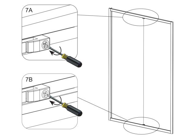
When fitting a fully framed product into a recess you must push the wall profiles on the uprights. Then lift the assmbled frame onto the tray.
