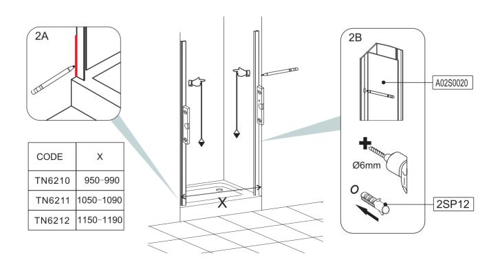
Fit your fixed panels seal to the top and bottom of the fixed panel.
