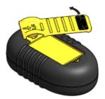
Remove the battery compartment cover and replace the battery. Alkaline Duracells are recommended.
