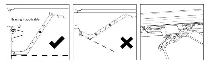
Once installed, prior to configurating your opener attach the stopping mechanism as shown below with your door in the fully opened position (refer below). This will avoid the carriage overrunning during limit and force settings.
