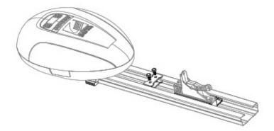
Using screw M6.3\*20 fix the track with motor head through the U shaped buckle for added strength to ensure the mechanism doesn't move.
