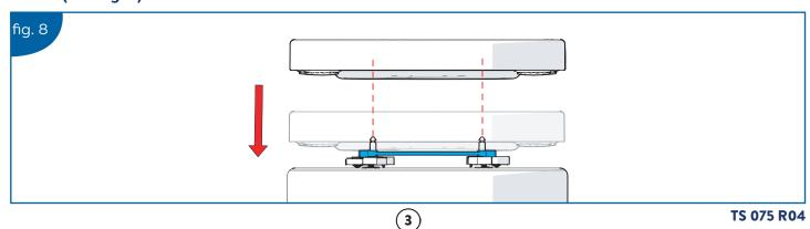
Align the seat with your toilet pan by rotating and sliding the flexi fix brackets (B). If required, lift the seat off the pillars to help with the adjustment. (See Fig. 9)
