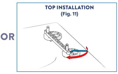
Remove the spacer from the flexi fit brackets
