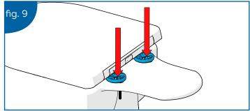
Carefully remove the seat **without disturbing the bracket positions** and fully tighten the screws (J) to firmly secure the hinge brackets. **(See Fig. 10 and 11). Do not to over-tighten.**
