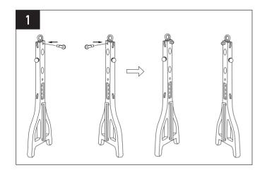
INSERT EYE PINS INTO TOP OF PILLARS AS SHOWN.
