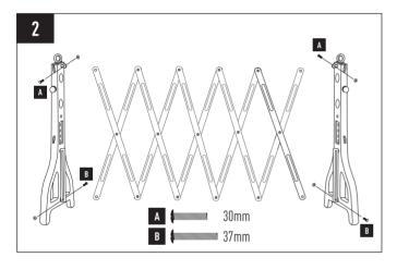
SECURE CONCERTINA SECTION TO TOP AND BOTTOM OF PILLERS USING THE NUTS, WASHERS AND BOLTS PROVIDED.
