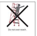
In proper use the platform is stable. Operatives should be instructed not to lean over the rail. Operatives should stand central to the top platform and work within arms distance of products or maintenance etc.
