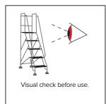
Complete visual checks before use – make sure there is no obvious damage to the structure of the steps. Checks should specifically look for: welds are structurally sound and no signs of distortion, wheels and or castors are in good condition and not damaged, foot pads are in position and in good order, tread material is in position and still adhered to the steel formed tread, the formed tread is still in good condition and not buckled.
