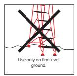
Use only on firm level ground. Surface should be sound and smooth – rough /uneven surfaces could cause the steps to be unstable. Moving the steps around on rough/uneven ground could also cause damage to the castors and footpads.
