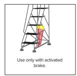
If not a spring-loaded step, then the brake bar must be in the retracted position prior to ascending the steps – i.e: the step must not be in the mobile mode where all 4 castors/wheels are in contact with the ground.
