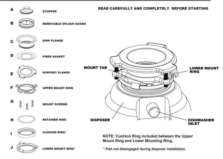
**NOTE:** As the mounting assembly is properly assembled at the factory, please pay close attention to the order of the mounting system parts.
