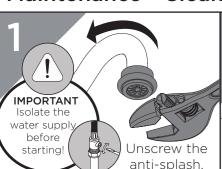
Remove the anti-splash and filter from housing.
