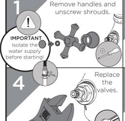
Remove the valves using a suitable spanner.
