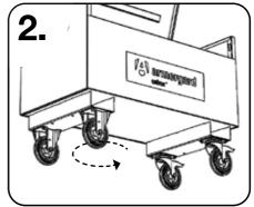
Repeat for the other 3 wheels. Once complete, check all nuts are tight, and then ensure the two braked castors can swivel 360° before lowering the OxBox.
