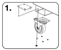
Only the OX3 and OX4 can be fitted with castors. Lift the box onto a stable platform, and then insert castor plates into the forklift skids. Put the castor wheel in place and use a 13mm socket to tighten the M8 nylocks.
