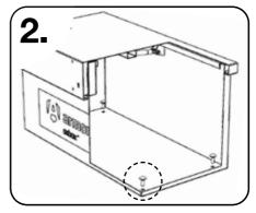
The OxBox should then be fixed down using four M10 bolts, washers, and shear nuts. The OxBox needs to have a bolt in each of it's four corners fixing it securely to the floor.
