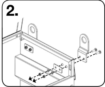
2. Thread the M10 coach bolts through the lifting eyes, then through the box. Inside the box add a backing plate, M10 washers and nylocks to each bolt as shown.
