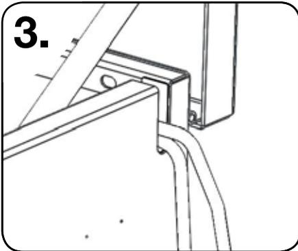
**3.** Up to 2 cables can be fitted into the cable pass-through, so a power supply and a tool can be fitted through simultaneously. The lid can then be closed and locked for secure charging.
