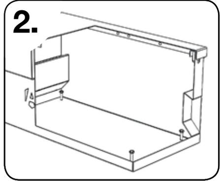
The TuffBank **MUST** then be fixed down using four M10 bolts, washers, and shear nuts. The TuffBank needs to have a bolt in each of it's four corners fixing it securely to the floor.
