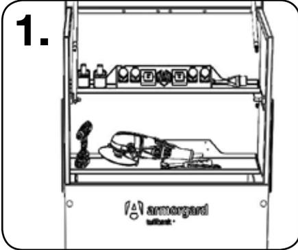
**1.** With a PowerShelf fitted to your TuffBank, you can charge batteries and mobile devices, or power tools while keeping them secure. **WARNING:** Ensure you read the safety information at the beginning of this manual before use.
