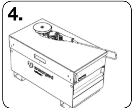
**4.** Remember that only the keyholder can access the PowerShelf, so ensure that any tools or items are unplugged once finished with to reduce risk from electrical hazards.
