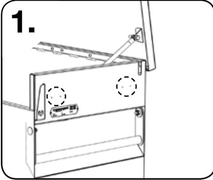
1. All TuffBanks except TB1, TB12 & TB21 can be fitted with crane lifting eyes. To fit the kit, use a 10mm metal drill bit to drill out the 4 pilot holes located on each side of your TuffBank.
