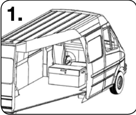
To install a TuffBank in a vehicle, these instructions **MUST** be followed. The installer must drill 4x 10mm holes into the box, one in each corner, in order to fix it to the floor.
