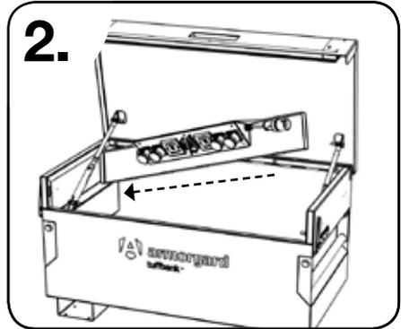
Slide the left end of the shelf into the TuffBank, under the gas strut with the SlamStop safety stay.
