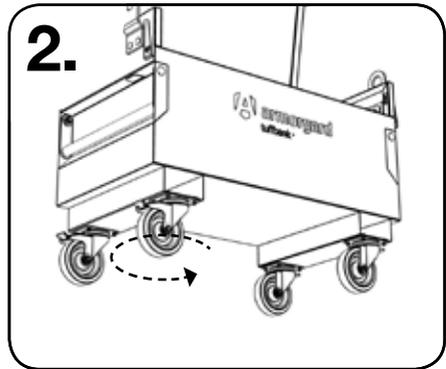
2. Repeat for the other 3 wheels. Once complete, Check all nuts are tight, and then ensure the two braked castors can swivel through 360° before lowering the TuffBank.
