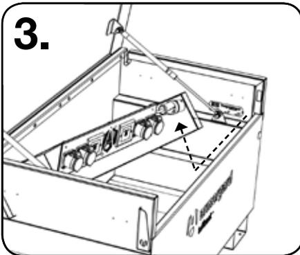
Slot the right hand side of the shelf down in front of the gas strut, bring it underneath, and back up behind the gas strut.
