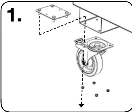
1. All TuffBanks except TB1 & TB12 can be fitted with castors. Lift the box onto a stable platform, and then insert castor plates into the forklift skids. Put the castor wheel in place and use a 13mm socket to tighten the M8 nylocks.
