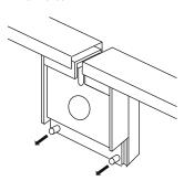
2 Locate the keyhole and the 4 holes on the back of the disc lock and blow all dust and dirt out the lock using a compressor or a pressurised canister.
