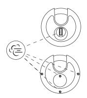
3 Lubricate lightly in the 4 small holes and the key hole. We recommend using a lubricant spray that contains PTFE additives for the best performance.
