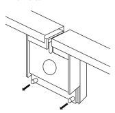
2 Locate the keyhole and the 4 holes on the back of the disc lock and blow all dust and dirt out the lock using a compressor or a
