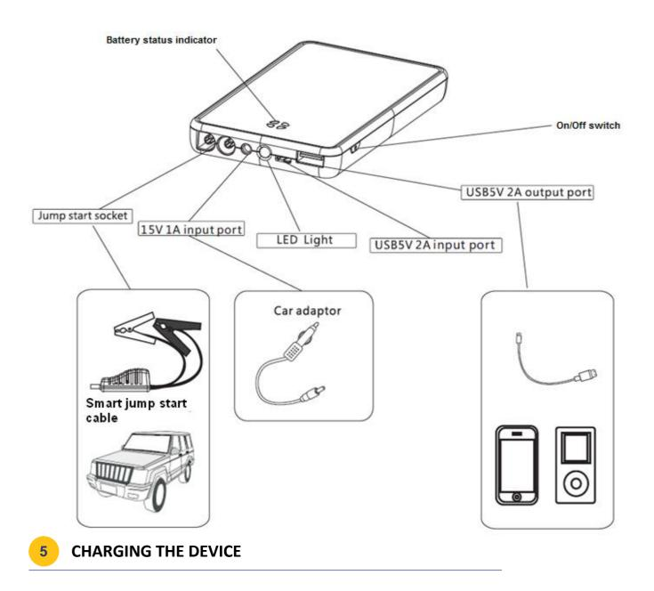
Depressing the switch on the side of the unit will result in the blue LED segments on the face of the device to illuminating. The number of segments which alight signifies the current level of charge within the device:
