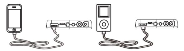
Connect the device you wish to be charged to the USB socket using an appropriate cable and momentarily depress the button on the side of the unit. The blue battery status LEDs on the face of the product will illuminate and charging will commence automatically.
