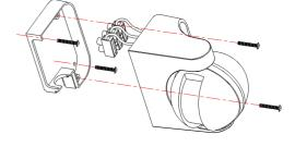
Put the sensor on the bottom lid, twist the screw tightly then electrify it and test it.
