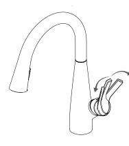
1.Pull the handle out to, turn on and to control the flow.
