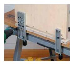
... first switch the board clamp from the left corner to the right. Only then, slide the drill guide to the last hole to be bored.
