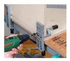
Then drill both the face hole into the shelf bottom and the hole into the side wall.
