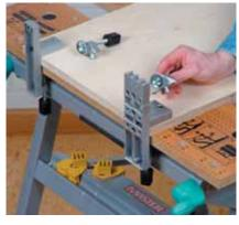
Screw the shelf bottom tight to the workbench with the Universal Dowelling Jig and insert the two clamp supports.
