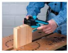
Position the Dowelmaster on a dowel, slide the angle fence against the side of the board, and tighten the screw.
