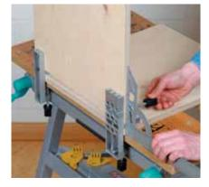
Insert the side wall into the dowelling jig, match the wood edges precisely to each other with an angle, and clamp them tight.
