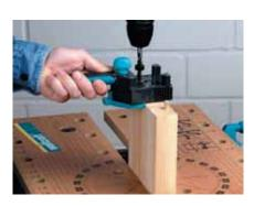
Clamp the two boards into the workbench. Slide the Dowel-master with the guide groove over the dowel, and drill.
