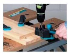
Clamp the face board board with the dowels on to the board that is to be drilled and slide the Dowelmaster with the guide groove over the dowel. The fence then butts firmly against the lower edge of the board.
