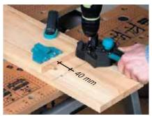
Mark the centre of the shelf on the side board and clamp the shelf at a distance of 40 mm.
