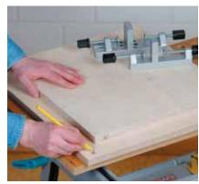
Mark all shelf bottoms with a cross on the edge and the side walls with a cross on the wood surface.
