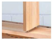
When T joints (e.g. for centre shelves) are to be made, the Dowelmaster is used without the angle fence.
