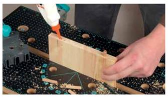
In order to be able to drill the counter-holes, the dowels must first be glued into the face holes.
