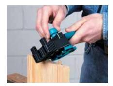
To adjust the fence of the Dowelmaster to the dowels already drilled, loosen the fastening screw and insert the dowels into the corresponding drill bush of the Dowelmaster.
