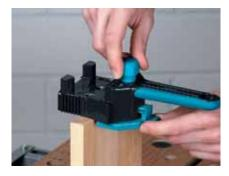
Then slide the fence firmly up against the side of the board and secure it with the fastening screw. Now the fence is precisely adjusted to the centre of the dowel and of the board.
