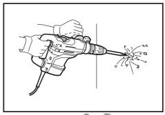
Set the change lever to the 1 or 7 symbol. Hold the tool firmly with both hands. Turn the tool on and apply slight pressure on the tool so that the tool does not bounce around, uncontrolled. Pressing very hard on the tool will not increase the efficiency.
