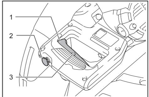
► 1. Switch trigger 2. Lock-off button 3. Hole for padlock
