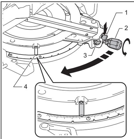
► 1. Lock lever 2. Grip 3. Releasing lever 4. Pointer
