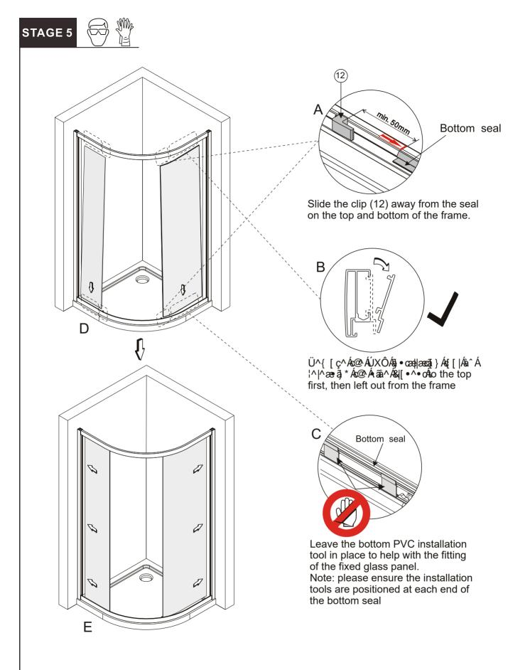
D. Standing inside the enclosure, place the bottom of the fixed panel on the frame at a slight angle, then lean the panel forward into the top of the frame.
