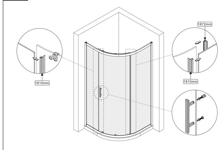
Adjust the rollers to ensure the the overlap of the moving and fixed panels is parallel.
