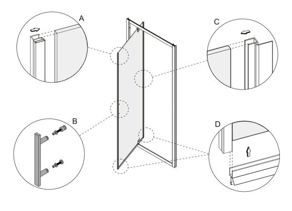
A.Loosen the bolt on the bottom pivot bracket, to insert the small seal, MB0081. Then fully tighten the bolt.
