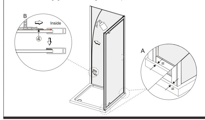
A. Adjust the door frame side to side until the side panel is parallel to the side of the tray and the top of the door panel is parallel with the frame.
