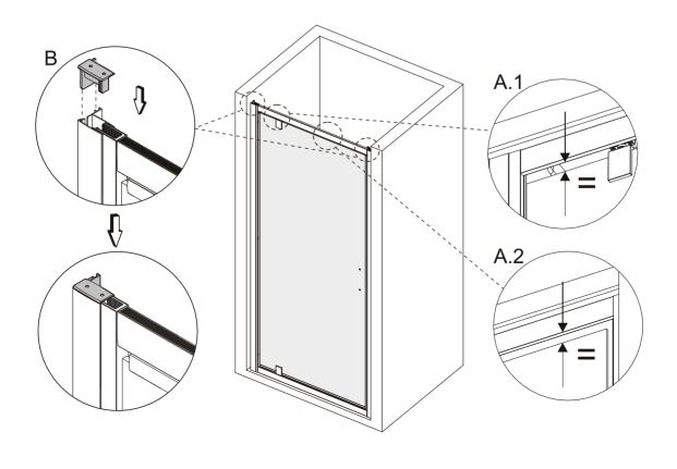
Push the wedge seals between the bottom profile and the tray to hold the frame in position. Three thicknesses are provided.
