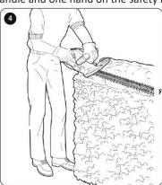
**TRIMMING NEW GROWTH** (Figure 5) - A wide, sweeping motion, feeding the blade teeth through the twigs is most effective. A slight downward tilt of the blade, in the direction of motion gives the improved cutting.
