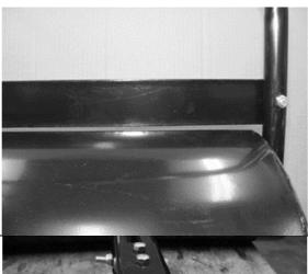
Fit the Scraper to the Drawbar assembly using the 40mm Coach Bolts and Nuts. Ensure that the scraper just clears the Roller before tightening the Nuts.
