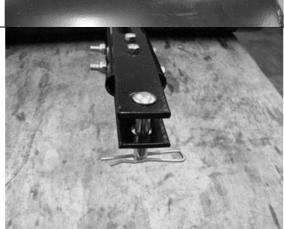
Insert the Towing Pin and secure with the R-Clip, as shown.
