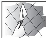
For multi-layered, painted-over or water-resistant wallpapers especially, we recommend working on the areas to be stripped using a wallpaper scorer in a grid pattern.
