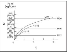
1. Fastening time (second) 2. Fastening torque
