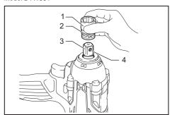
Impact socket 2. Hole 3. Square drive 4. Detent pin
