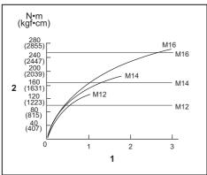
1. Fastening time (second) 2. Fastening torque
