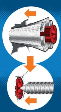
WET FIX° fills and bonds the gap making your wall plugs fit tight.
