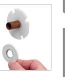
Trim the projecting pipe to a length of 15-22mm, measured from the face of the gripper ring, using a rotary type cutter. If a hacksaw is used, the pipe end must be carefully de-burred and chamfered.
