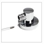
Ensuring the locking screw hole is positioned at the bottom, place the wall outlet mounting plate onto the pipe assembly and mark and prepare the fixing points, using the fixings provided, if suitable.
