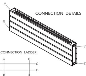
The standard connection configuration is ABCD. Same end connections require a baffle. Any non standard configurations should be specified at time of order
