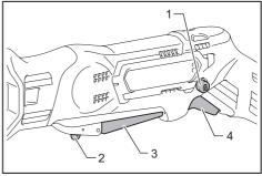
1. Lock-off button 2. Lock-off lever 3. Switch lever
