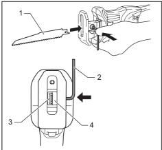
▶ 1. Recipro saw blade 2. Hex wrench 3. Hole for recipro saw blade 4. Blade clamp
