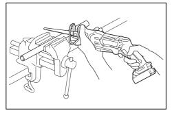
Press the shoe firmly against the workpiece. Do not allow the tool to bounce. Bring the recipro saw blade into light contact with the workpiece. First, make a pilot groove using a slower speed. Then use a faster speed to continue cutting.
