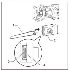
1. Recipro/jig saw blade 2. Blade clamp 3. Hole for recipro saw blade 4. Hole for jig saw blade
