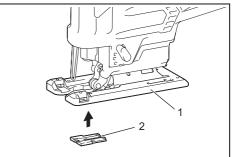
▶ 1. Base 2. Anti-splintering device
