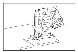
To trim edges or make dimensional adjustments, run the jig saw blade lightly along the cut edges.
