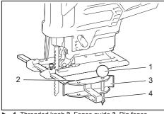
1. Threaded knob 2. Fence guide 3. Rip fence (Guide rule) 4. Pin
