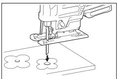
For internal cutouts without a lead-in cut from an edge, pre-drill a starting hole 12 mm or more in diameter. Insert the jig saw blade into this hole to start your cut.
