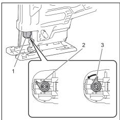
Jig saw blade holder 2. Released position
