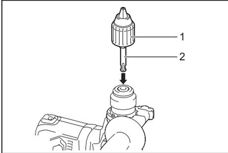
► 1. Drill chuck assembly 2. Chuck adapter
