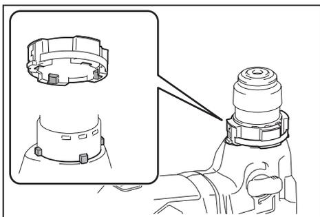
Install the side grip (optional grip base set and standard grip) so that the groove on the grip fit in the protrusion on the spacer. Turn the grip clockwise to secure it.
