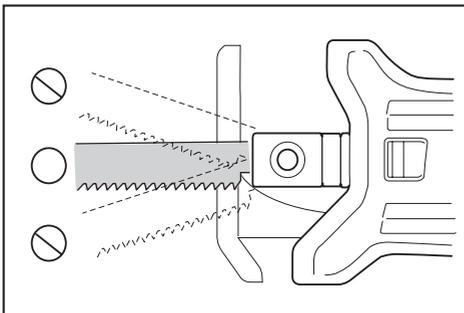
You can use both jig saw blades (B type) and reciprocating saw blades according to your work. Insert the reciprocating/jig saw blade straight into the blade clamp and tighten it by hex wrench. Pull the reciprocating/jig saw blade lightly to make sure that the reciprocating/jig saw blade does not fall off during operation.
