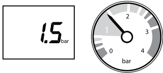
Fig.52 Restore water pressure
