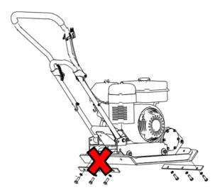
Attach the Paving Pad onto the front of the Base Plate as shown. Align the holes in the Base Plate, Paving Pad and Clamp Plates, and secure it with lock washers 10 and bolts M10x30.
