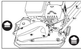
The unit must be transported in the upright position to prevent fuel from spilling. Do not lay the machine on its side or top.
