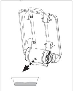
Remove the pipe plug from the top of the exciter housing. Tilt the housing upside down so that the oil drains from the exciter. Examine oil for metal chips as a warning of future issues. Return the plate housing to the upright position
