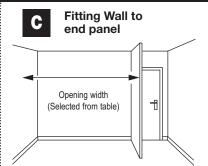
To stop the doors short of an obstruction such as a window or door, construct a return end panel from melamine faced chipboard. Cut to fit the exact ceiling height and scribe back edge to fit rear wall and skirting.
