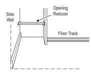
To reduce your opening by more than 457mm / 18" on each side you can construct an 'L' section using an end panel and end fillet.
