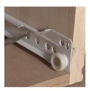
8. Along the length of the runner, there are 2 oval holes. Place the runner along at the marked position and insert 2 screws through the oval holes.
