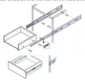
8. Secure the runner to the drawer using the supplied screws, making sure that the slides are the same height on both sides of the drawers.
