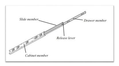
2. Separate the Cabinet Member from Drawer member using the Release Lever.
